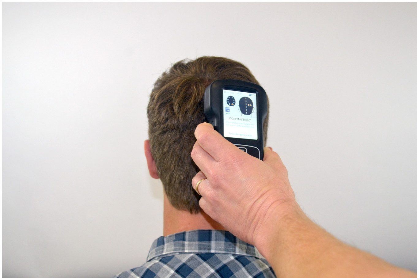
Figure 1 Infrascanner Model 2500 during scanning of the right occiput. Reproduced with permission from and provided courtesy of InfraScan (Philadelphia, PA).
